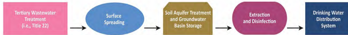
a) Indirect potable reuse using groundwater replenishment via surface spreading .
